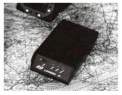
1993 – Electronic Barographs with GPS input. Two companies that had been producing electronic barographs, in 1993 developed versions with larger memory that could connect to a Garmin GPS receiver unit and record GPS fixes as well as pressure altitude. These companies were EW Avionics (UK, MD Wayne Richards) and Borgelt Instruments (Australia, MD Mike Borgelt).
